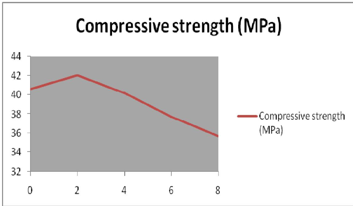
The variation of compressive strength of SCC containing foundry waste sand
