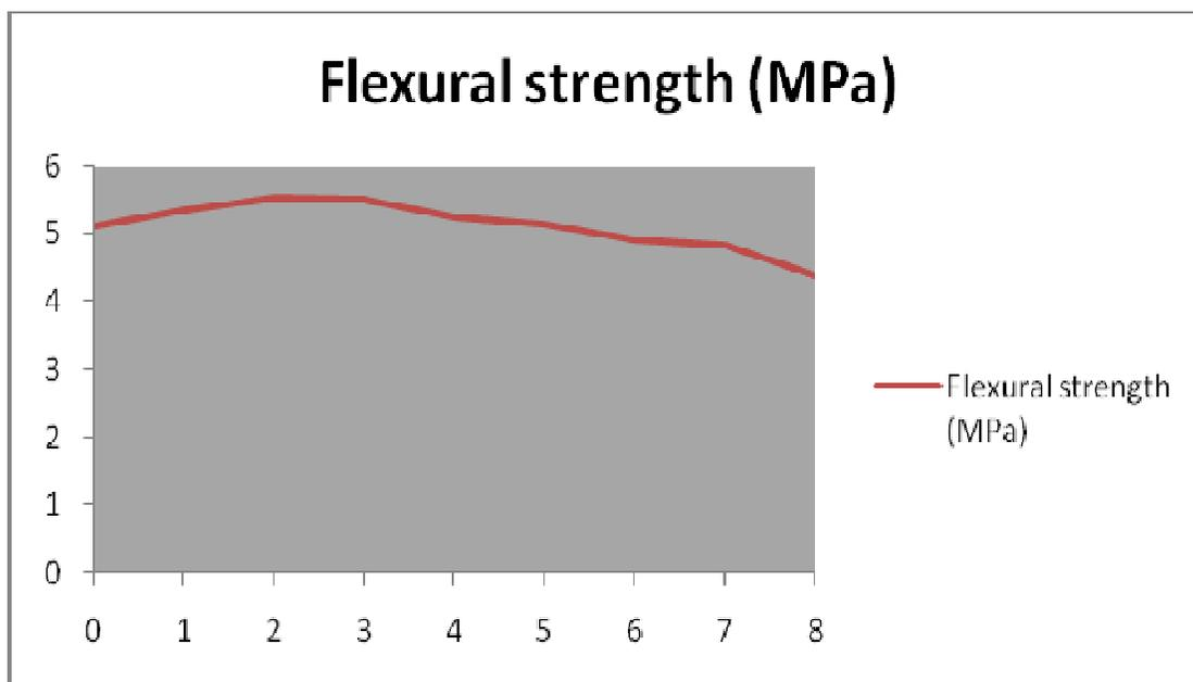
The variation of flexural strength of SCC containing red mud
