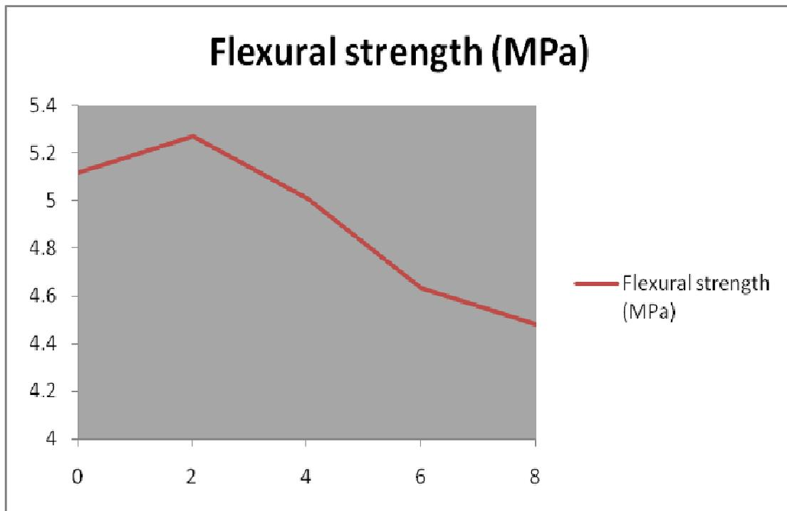
The variation of flexural strength of SCC containing red mud
