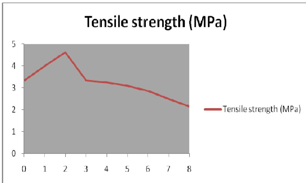
The variation of tensile strength of SCC containing red mud
