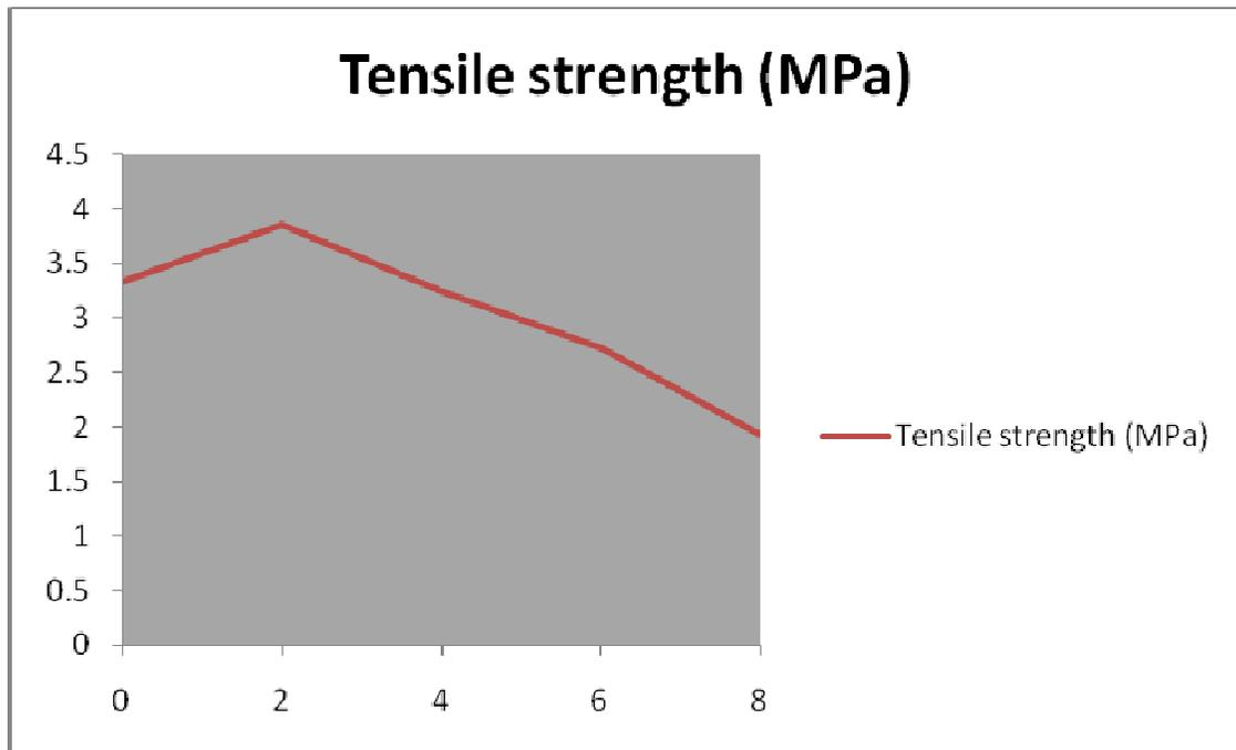
The variation of tensile strength of SCC containing foundry waste sand
