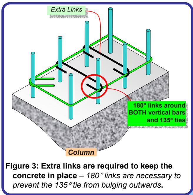
**Figure 3:** Extra links are required to keep the concrete in place –  $180^\circ$  links are necessary to prevent the  $135^\circ$  tie from bulging outwards.
