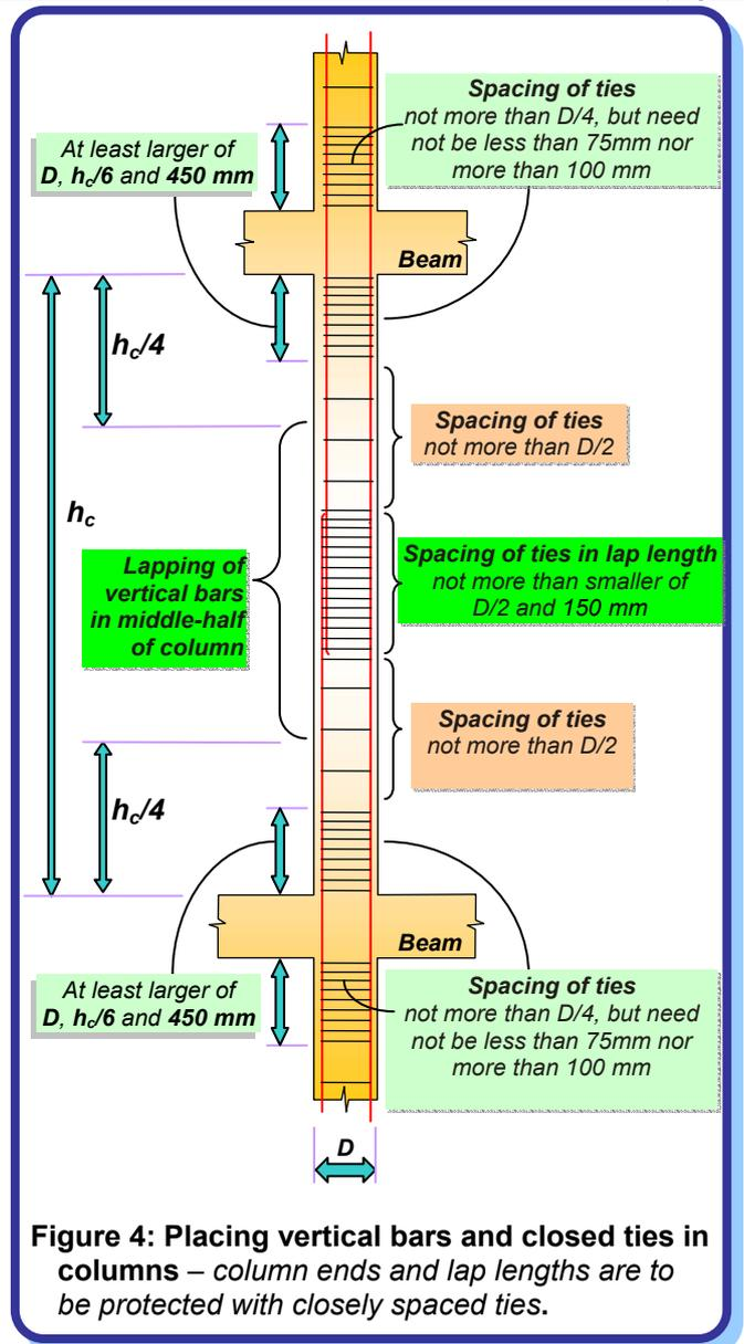
**Figure 4:** Placing vertical bars and closed ties in columns – column ends and lap lengths are to be protected with closely spaced ties.
