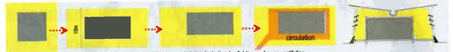
Budget and scale of building dictated a compact footprint which was made linear for better day lighting and cross ventilation. The inherent programmatic split, of core clinic functions, waiting areas and are arranged as 2 concentric layers creating a building within a building. A generous and airy waiting verandah wraps around the core hospital. An additional outdoor layer of varied cultivated landscapes further helps create an aesthetic climatic buffer that controls glare and dust.
